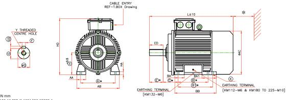
ALL DIMENSIONS ARE IN mm RINGED DIMENSIONS ARE AS PER IS:1231/IEC:60072-1 \*TOLERANCES ON MANDATORY DIMENSIONS ARE AS PER IS:1231/IEC:60072
