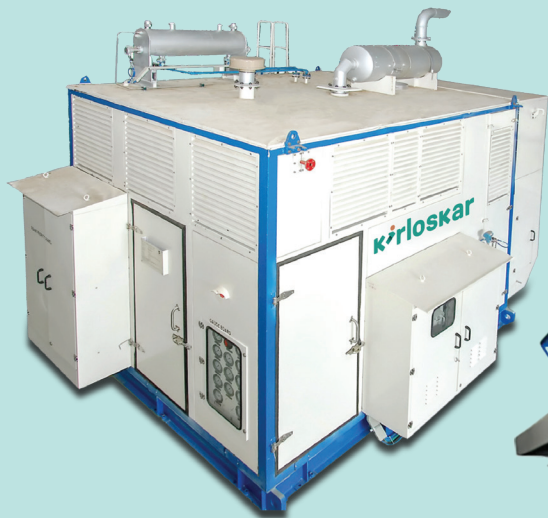
KCNG-OC Series Our Engine & Motor Driven CNG Packages are Suitable for Online CNG station. Capacity ranging from 400 SCMH to 3500 SCMH and suction pressure ranging from 0.55 barG to 70 barG
