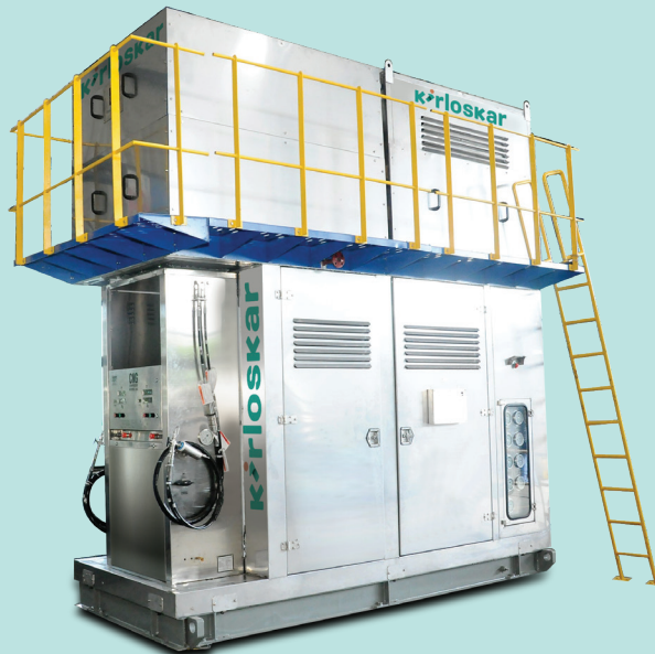
KCNG-IG Series Compact design where cascades and dispensing units are integrated in the compressor unit. Suitable for the stations where space is the challenge
