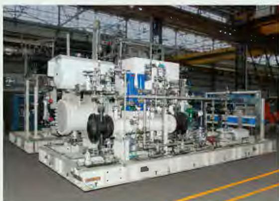
**Propylene Refrigeration Package for Sulphuric Acid Plant - Oil & Gas Sector**
