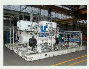
Propylene Refrigeration Package for Sulphuric Acid Plant - Oil & Gas Sector
